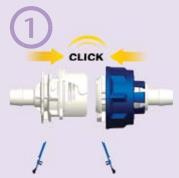
Align male and female couplings, push together until "Colder Click" confirmation. Slight rotation of lock ring may be required for proper alignment prior to connection.
