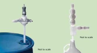
104 DrumQuik® 3-Port UDA: Used with 3/4" male NPT coupling terminations to adapt dip-tubes to standard drum closures for closed system dispensing. Material: Food grade, virgin polypropylene Thread Sizes: UDA 3-Port: 3/4" male NPT; UDA: none
