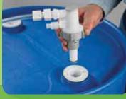
Turn the coupler locking ring-clockwise until stop is reached (approximately 2 full turns); valve is opened during this process.
