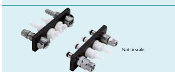
**70** Multi-Mount: Connects three to five lines at once; keyed to prevent mismatched connections. Material: Acetal, chrome-plated brass Tubing ID Sizes: 1/8" to 3/8" (3.2mm to 9.5mm)
