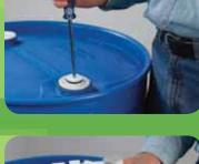
4 Insert coupler into drum insert assembly.
