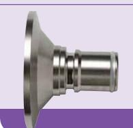
**82** SaniQuik<sup>TM</sup>: Integral sanitary termination attaches to hard-plumbed systems with sanitary clamps; permits quick and easy connection to single-use bag systems, manifolds or tube sets with MPC or MPX bodies. Material: 316L stainless steel
