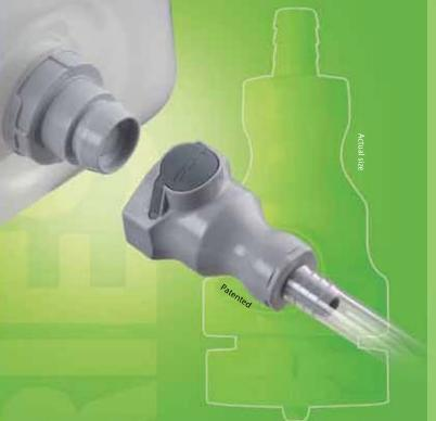
The patented 3/8" flow Universal Dispensing Coupler (UDC) provides a universal connection to a 38mm threaded or snap-in fitment neck. Make instant connections to bulk packaging systems including bag-in-box (BIB), flexible and rigid packaging styles. Automatic flush face valves minimize costly or dangerous spillage. An ergonomic design and a large, shrouded thumb latch pad produce a coupling that is easy to grip and simple to operate.
