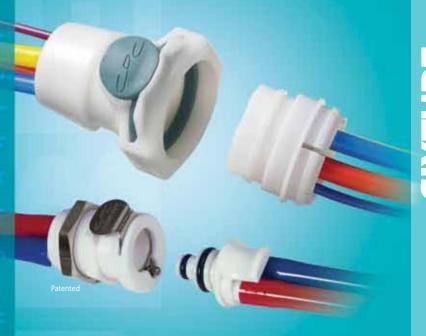
The Sixtube<sup>TM</sup> coupling provides one easy-to-use guick disconnect for up to six separate fluid lines. The Sixtube is available with valves on either side for maximum design flexibility. Featuring the Colder thumb latch, the Sixtube can disconnect up to six lines with the push of a button. The snap-in panel mount design keeps a low profile on the front of the equipment panel.
