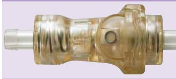
**84** HFC39: Features aseptic disconnect functionality with automatic shutoff valves, preventing external organisms from entering the media flowpath upon disconnection. Material: Medical-grade polysulfone Tubing ID Sizes: 1/4", 3/8" and 1/2" (6.4mm, 9.5mm and 12.7mm)
